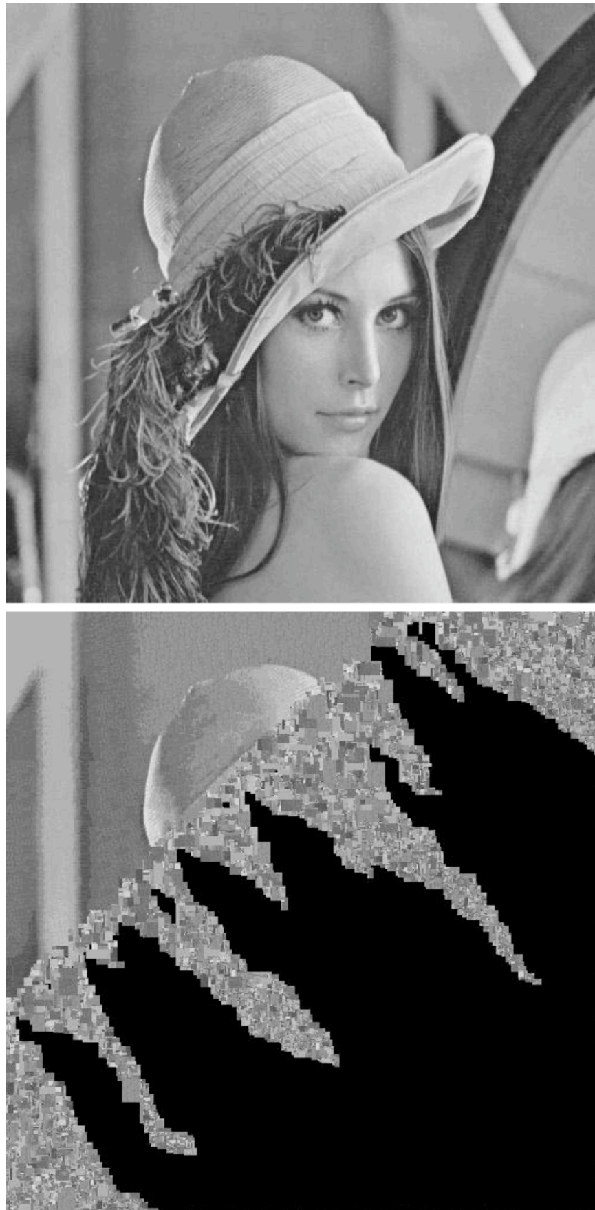
Fig.4: Lena original image and Lena decompressed after 1 byte in the input stream has been corrupted
