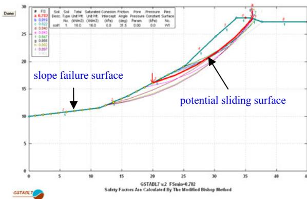
Figure 5. Slope failure surface at 13k+730.
