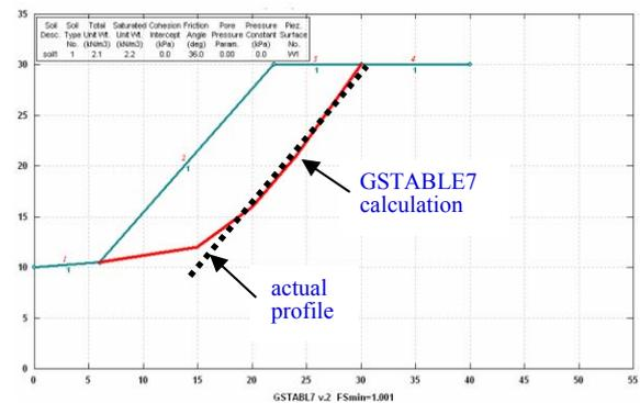
Figure 6. Comparison of result at 18k+650.
