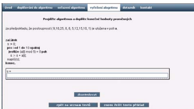
Fig.19 Web application “algds” - Solve the given algorithm (i.e. determine the value of the variable s )
