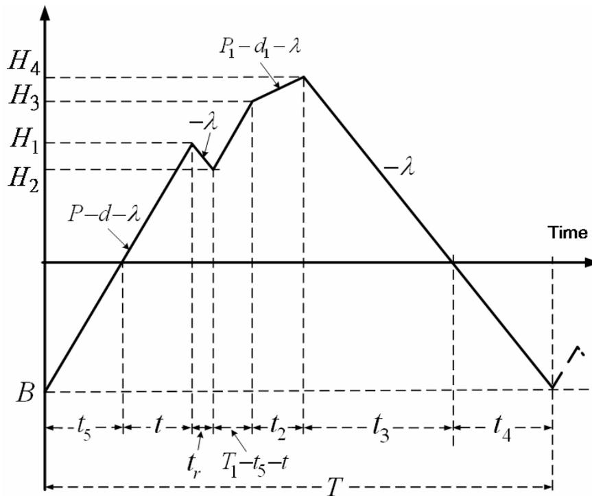
**Fig.1:** On-hand inventory of perfect quality items in EMQ model with failure-in-rework and breakdown happening in stock-piling time
