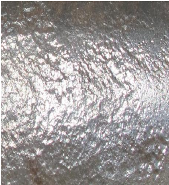
Figure ۳.۴ - initially a layer of coating with a thickness of ۳۰ microns was placed on surface of a piece of pipe with referred standard. Left figure two layers of ۳۰ microns (thickness ۶۰ microns) was placed on the surface.
