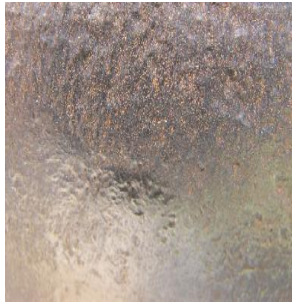
Figure ۳.۴ - initially a layer of coating with a thickness of ۳۰ microns was placed on surface of a piece of pipe with referred standard. Left figure two layers of ۳۰ microns (thickness ۶۰ microns) was placed on the surface.
