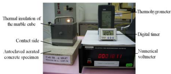
Fig. 2. Contact temperature measuring at the surface of autoclaved aerated concrete specimen with a relative moisture content of 6.35%
