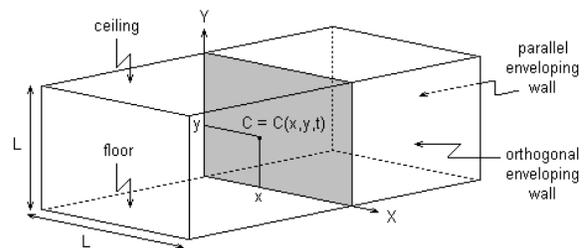
Fig. 1. Two-dimensional domain for simulations ( $xy$ -plane in a closed room or test chamber).
