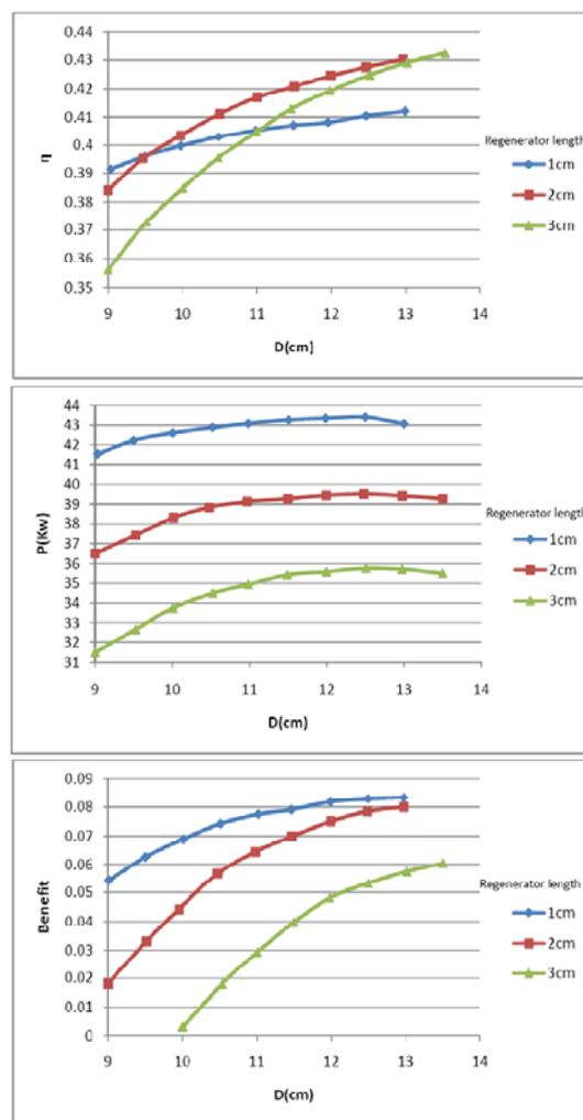
Fig. 9. Optimization of L and D ( $d_w=0.05$  mm)
