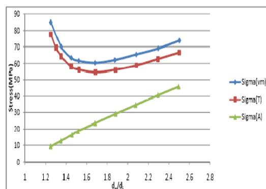
Fig.3. Stress variation with diameter ratio
