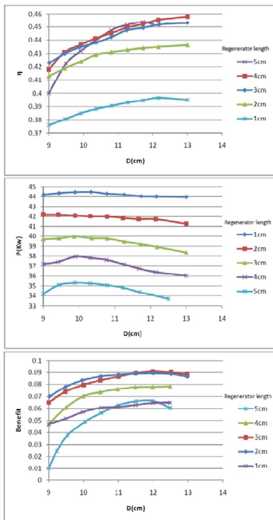
Fig.8. Optimization of L and D ( $d_w=0.1$  mm)
