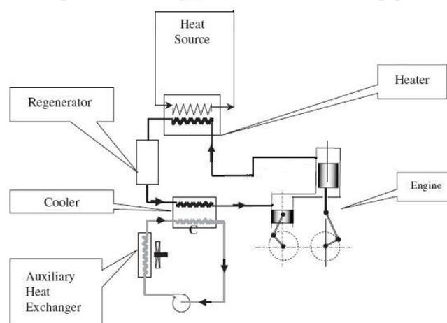
Fig.2. Heat exchangers in Stirling Engine
