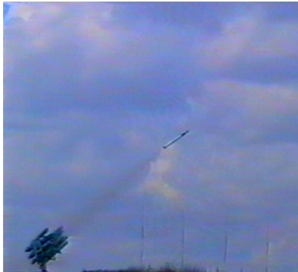
Fig. 15 Shooting test of anti-hailstone rocket
