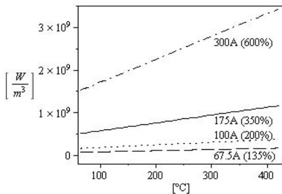
Fig.15. Heat produced by electrical current  $F_1$
