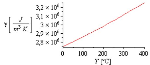
Fig.12. Heat capacity of zinc (per volume)
