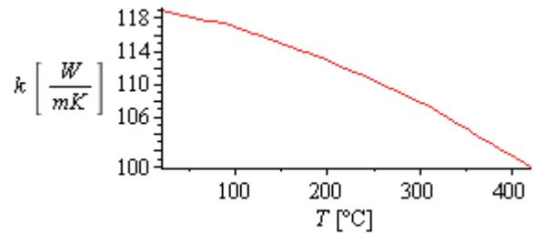
Fig.11. Heat conductivity of zinc
