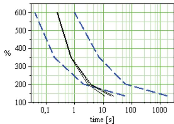
Fig.16. 50A Fuse time-current curve
