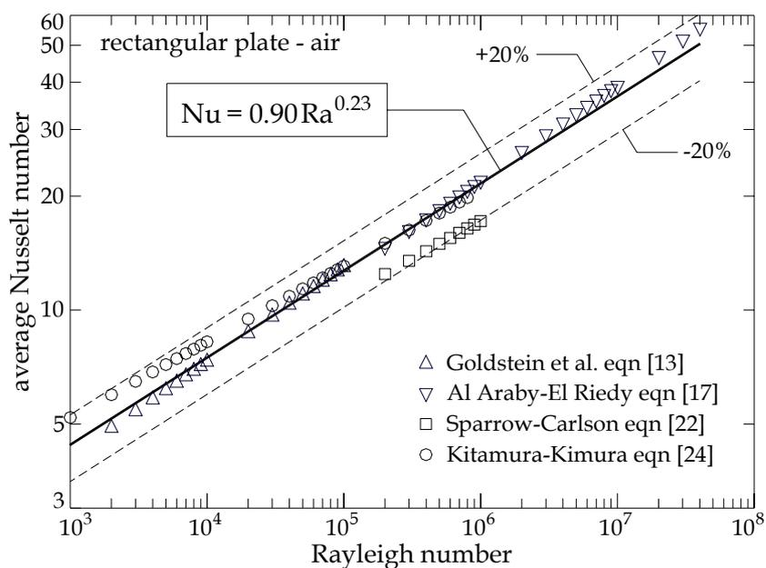
Fig. 2. Rectangular plates in air: literature data and mean heat transfer correlation.
