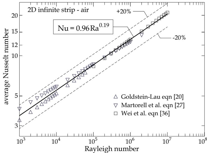
Fig. 3. 2D infinite strips in air: literature data and mean heat transfer correlation.
