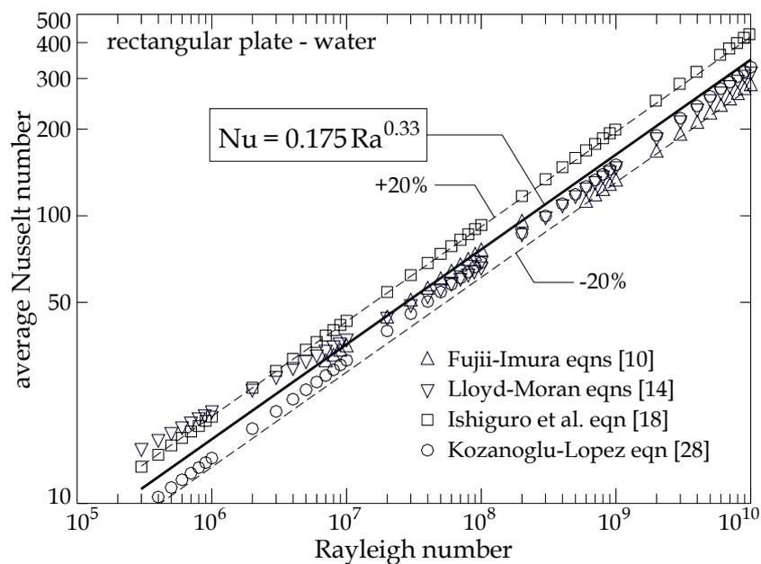
Fig. 4. Rectangular plates in water: literature data and mean heat transfer correlation.
