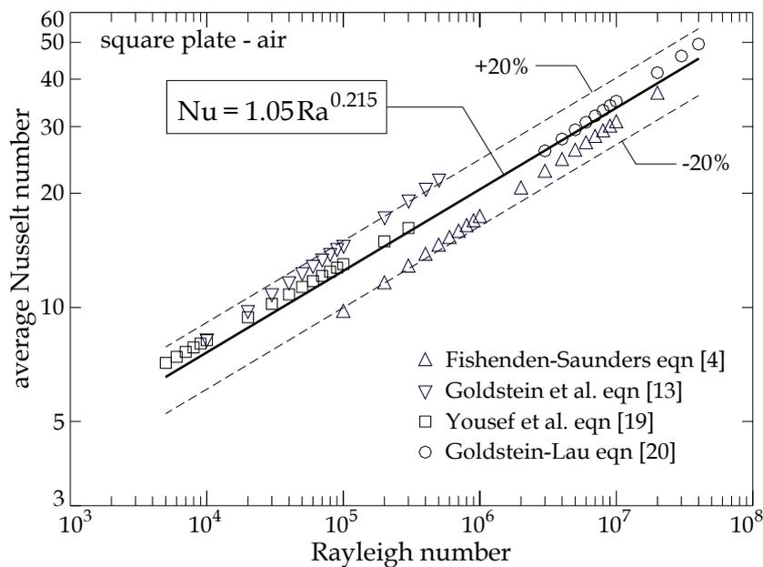
Fig. 1. Square plates in air: literature data and mean heat transfer correlation.
