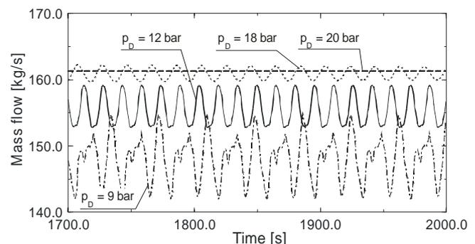
Fig. 7: Mass flow in the downcomer at different drum pressures
