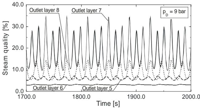
Fig. 8: Steam quality at the outlet of the four tube paths at a drum pressure of 9 bars
