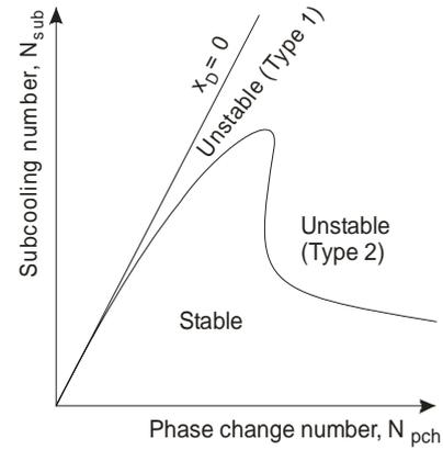
Fig. 1: Schematically stability diagram for DWO [26]
