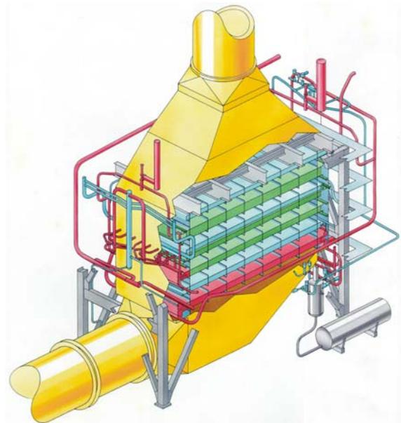
Fig. 2: Sketch of a vertical type HRSG [27]
