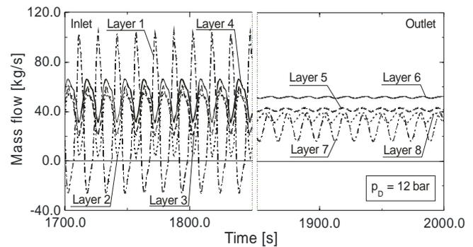
Fig. 6: Mass flow at the inlet of the layers 1 to 4 and at the outlet of the layers 6 to 8
