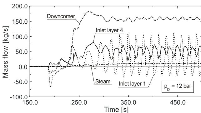
Fig. 5: Mass flow in selected tubes of the HRSG
