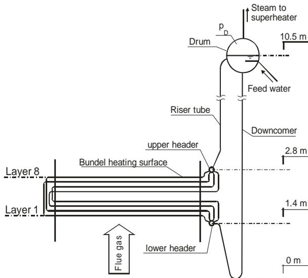
Fig. 3: Sketch of the simulated evaporator of the natural circulation HRSG
