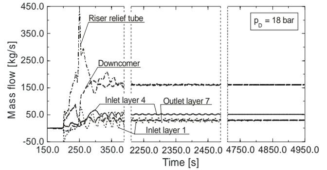
Fig. 9: Mass flow in selected tubes of the HRSG at a drum pressure of 18 bars
