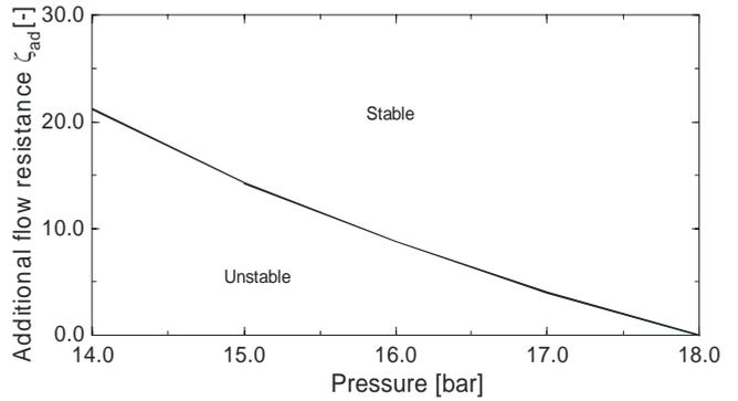
Fig. 11: Stability map for the additional flow resistance at the tube path inlet
