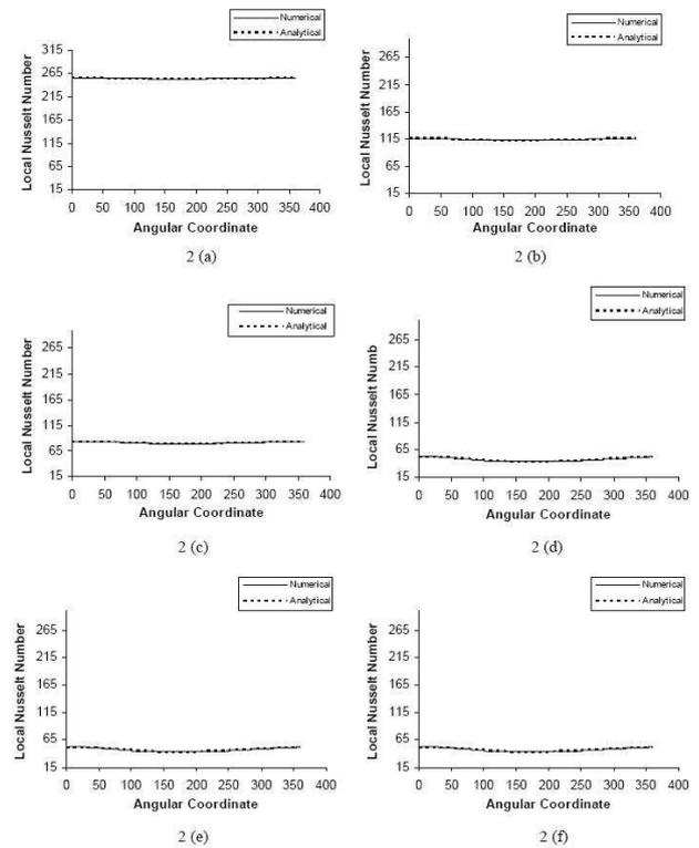
Figure 2: Local Nusselt Number comparison for  $Ri=0.0$ ,  $Re=1000$ ,  $K = 0.0$ ,  $\Omega = 0.25$ ,  $V = 1$  at times (a)  $t = 0.01$ , (b)  $t = 0.05$ , (c)  $t = 0.1$ , (d)  $t = 0.3$ , (e)  $0.5$ , and (f)  $t = 1.0$
