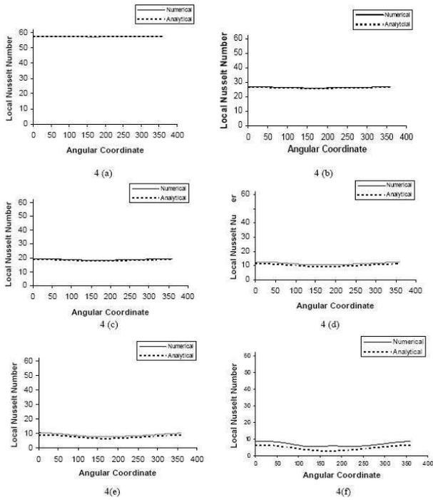
Figure 3: Local Nusselt Number comparison for  $Ri=0.0$ ,  $Re=50$ ,  $K=0.0$ ,  $\Omega=0.25$ ,  $V=1$  at times (a)  $t=0.01$ , (b)  $t=0.05$ , (c)  $t=0.1$ , (d)  $t=0.3$ , (e)  $0.5$ , and (f)  $t=1.0$
