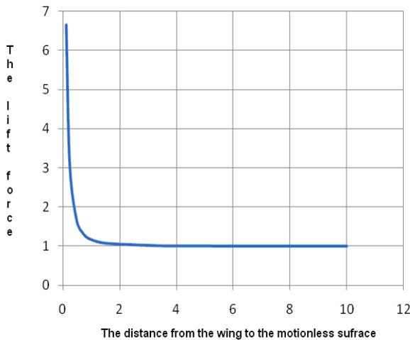
Fig.4 Dependence of dimensionless lift force of a flat wing  $\frac{F}{\pi\rho_0 \frac{V_0^2 \gamma}{\alpha} L}$  on the relative distance from the wing to the flat surface  $\frac{h}{L}$
