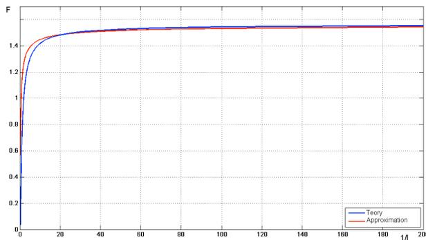
Fig.9 Relation between the force  $F_x$  and dimensionless parameter  $1/l$  obtained numerically and using approximation formula in case flow separation from the bottom of the body having singularity on the front edge.
