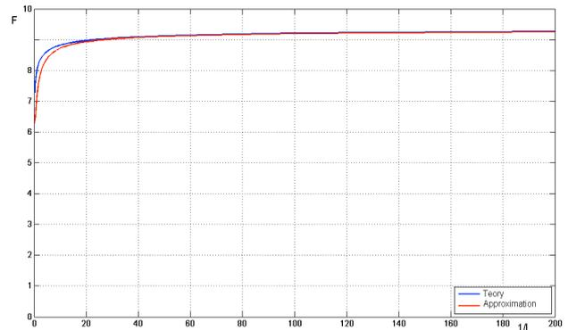
Fig.8 Relation between the force  $F_X$  and dimensionless parameter  $1/l$  obtained numerically and using approximation formula in case flow separation from the upper side of the body having singularity on the front edge.
