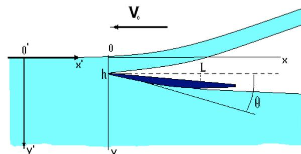
Fig.2 Schematic picture for thin wing motion near free surface with positive angle of attack
