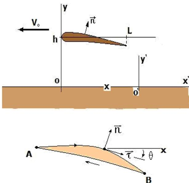
Fig.1 Schematic picture for thin wing motion above rigid surface
