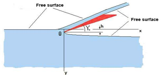
Fig.3 Schematic picture for thin wing motion near free surface with negative angle of attack
