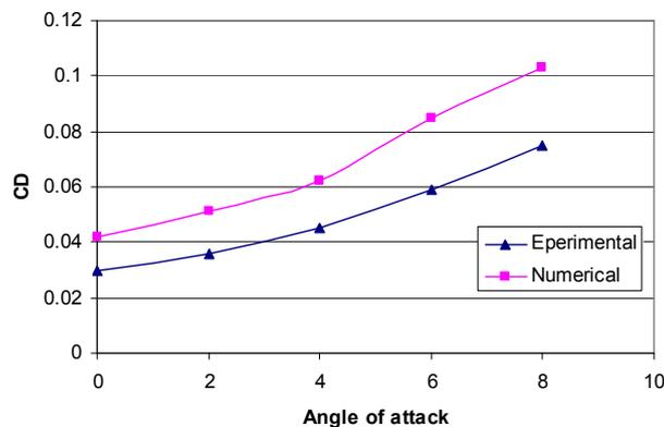
Fig.8 Drag coefficient versus angle of attack for  $h/c= 0.3$  and  $AR = 1.5$ .
