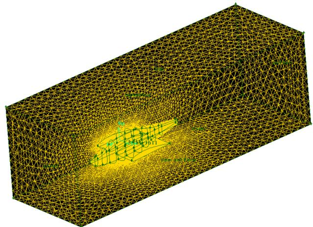
Fig. 3 The meshing of simulation for wing with hulls of WIG Catamaran.
