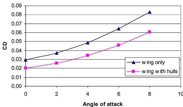
Fig.14 Drag coefficient versus angle of attack for h/c=0.4 for wing only and wing with influence twin hulls of WIG Catamaran.
