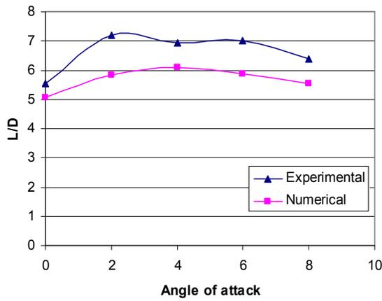
Fig.10 LIFT TO DRAG RATIO versus angle of attack for h/c= 0.3 and AR = 1.
