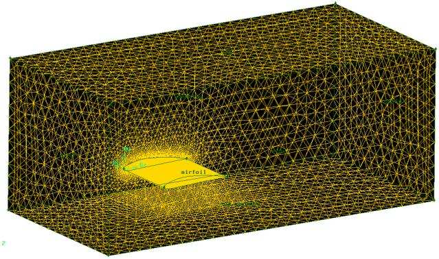
Fig. 2 The meshing of simulation for wing only.
