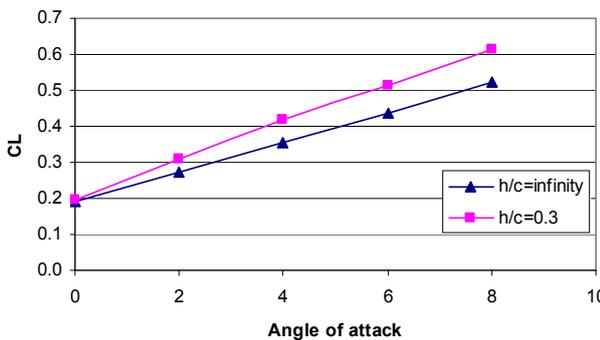
Fig.16 Lift coefficient for wing with influence twin hulls of WIG Catamaran versus angle of attack for  $h/c = 0.3$  and infinity.
