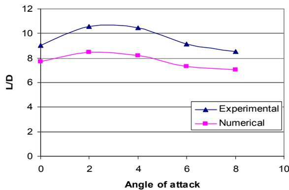
Fig.11 LIFT TO DRAG RATIO versus angle of attack for h/c= 0.3 and AR = 1.5.
