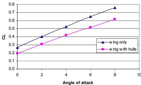
Fig.13 Lift coefficient versus angle of attack for h/c=0.4 for wing only and wing with influence twin hulls of WIG Catamaran.
