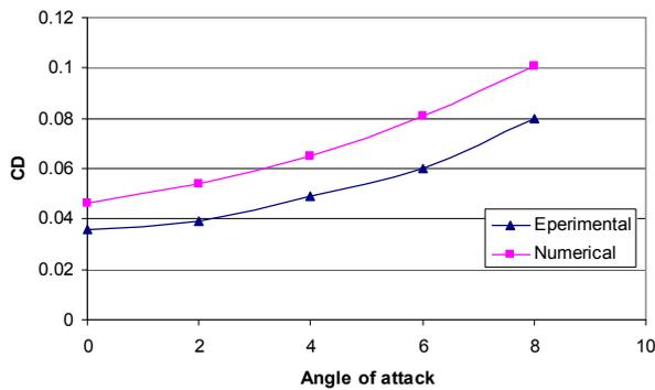
Fig.7 Drag coefficient versus angle of attack for  $h/c= 0.3$  and  $AR = 1$ .
