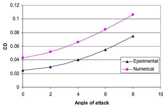
Fig.9 Drag coefficient versus angle of attack For  $h/c = 0.3$  and  $AR = 2$ .
