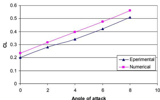
Fig.4 Lift coefficient versus angle of attack for  $h/c = 0.3$  and  $AR = 1$ .
