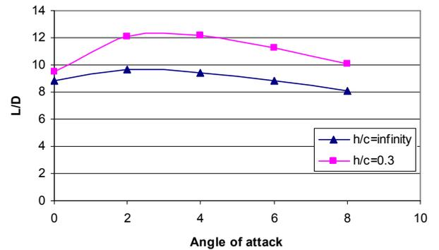
Fig.18 Lift to drag ratio for wing with influence twin hulls of WIG Catamaran versus angle of attack for  $h/c = 0.3$  and infinity.
