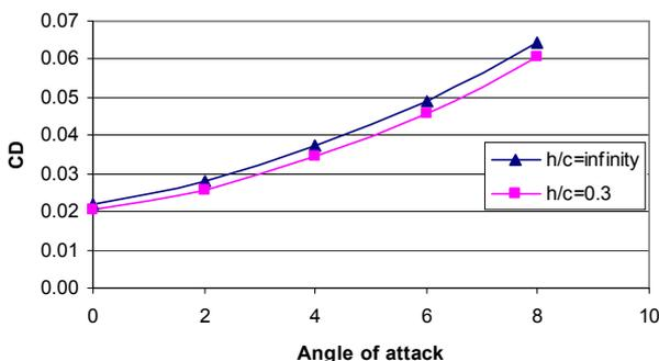
Fig.17 Drag coefficient for wing with influence twin hulls of WIG Catamaran versus angle of attack for  $h/c = 0.3$  and infinity.
