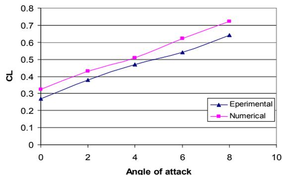
Fig.5 Lift coefficient versus angle of attack for  $h/c = 0.3$  and  $AR = 1.5$ .
