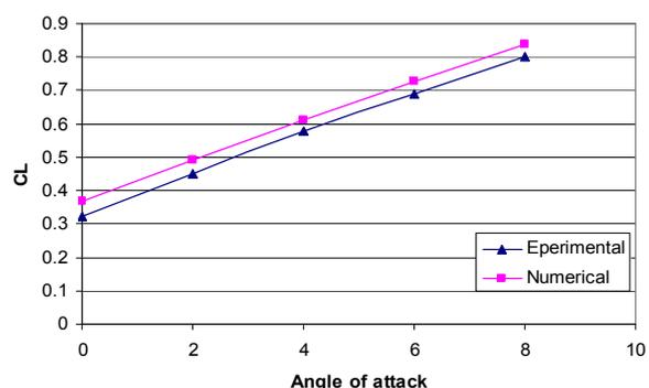
Fig.6 Lift coefficient versus angle of attack for  $h/c = 0.3$  and  $AR = 2$ .
