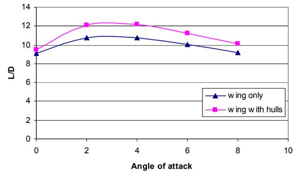
Fig.15 Lift to drag ratio versus angle of attack for h/c=0.4 for wing only and wing with influence twin hulls of WIG Catamaran.
