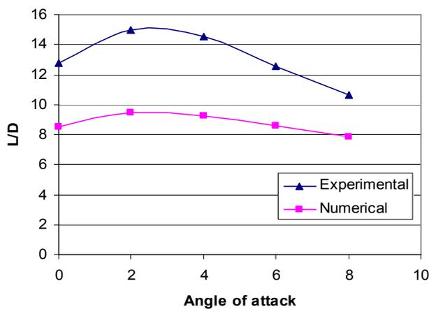
Fig.12 LIFT TO DRAG RATIO versus angle of attack for h/c= 0.3 and AR = 2.
