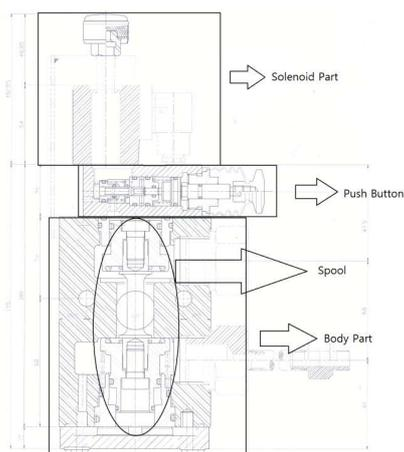
Fig. 1 Schematic diagram of 3/2 way solenoid valve
