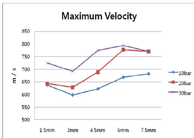
Fig. 9 Dependence of Maximum velocity on the spool displacement
