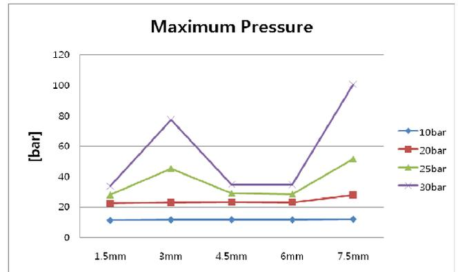
Fig. 12 Dependence of Maximum pressure on the spool displacement
