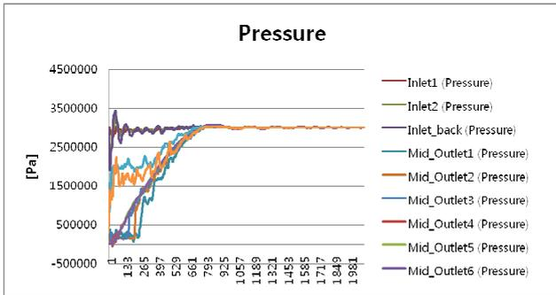
Fig. 11 Stabilization of pressure with respect to ime
