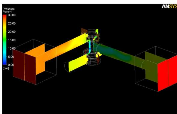
Fig. 18 Pressure at the outlet wall at 0.05s (Sin(t) graph case)
