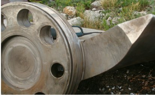
Fig.1 The cracked runner blade
