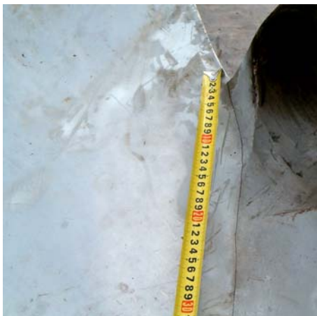
Fig.2 The crack on the pressure side
