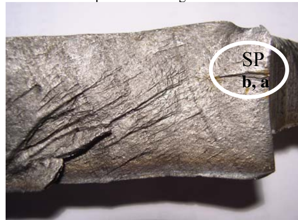
Fig.4 Macrograph of the fracture surface
