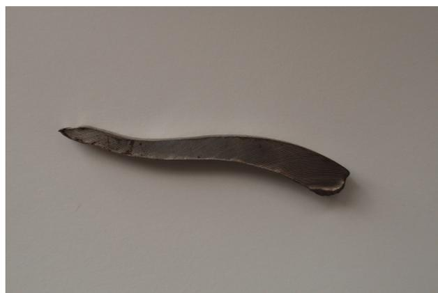
Fig. 6. View of the constant strength blade deformed by centrifugal force
