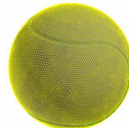
Fig. 7: CAD model with Tetrahedral mesh
