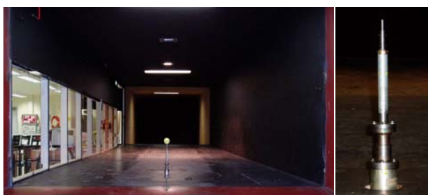
Fig. 2: A front view of experimental set up in RMIT Industrial Wind tunnel with a motorised supporting device (right)
