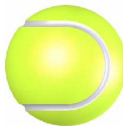
Fig. 6: 3D CAD model of tennis ball with 5 mm seam width
