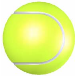
Fig. 5: A 3D simplified CAD model of tennis ball with 2 mm seam width
