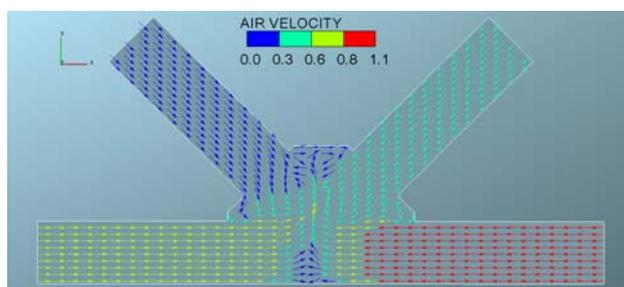
Fig. 6a Velocity vectors on a horizontal plane through the centre of tunnels, exit through 20 cm holes (empty bin scenario)
