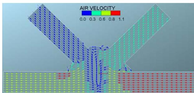
Fig. 6b Velocity vectors on a horizontal plane through the centre of tunnels, exit through top of tippel (empty bin scenario)
