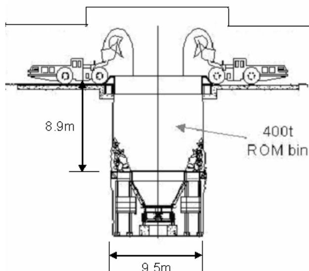
Fig.1 Typical LDH trucks tipping into a ROM bin
