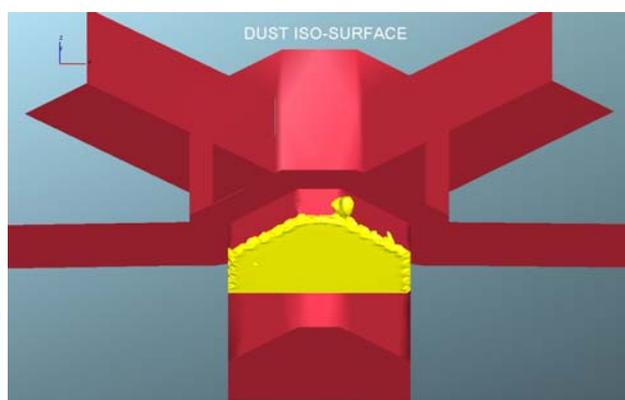
Fig. 7a Dust iso-contours or iso-surface ( $100 \text{ mg/m}^3$ ) (A snap shot of transient/time dependent case), exit through 20 cm holes (empty bin scenario)
