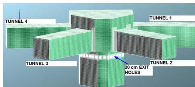
Fig.3 A typical computational grid used, exit through 20 cm holes (empty bin scenario)
