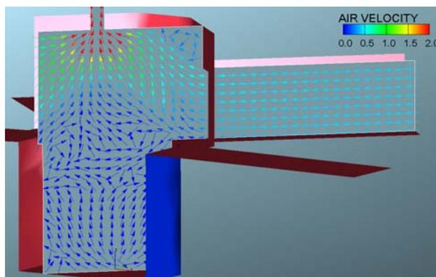
Fig. 5d Velocity vectors on a vertical plane through the centre of Tunnel 3, Exit through top of tippel (empty bin scenario)
