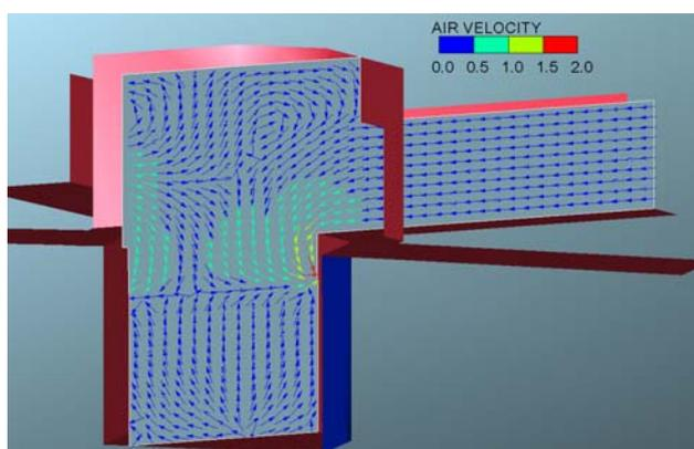
Fig. 5b Velocity vectors on a vertical plane through the centre of Tunnel 3 (empty bin scenario), exit through 20 cm holes (empty bin scenario)
