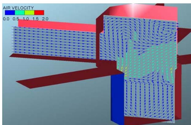
Fig. 5a Velocity vectors on a vertical plane through the centre of Tunnel 2 (empty bin scenario), exit through 20 cm holes (empty bin scenario)
