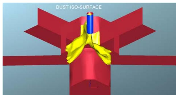
Fig. 7b Dust iso-contours or iso-surface ( $100 \text{ mg/m}^3$ ) (A snap shot of transient/time dependent case), exit through top of tippel (empty bin scenario)
