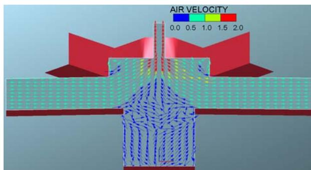
Fig. 4b Velocity vectors on a vertical plane through the centre of Tunnel 1 & 4, Exit through top of tipple (empty bin scenario)
