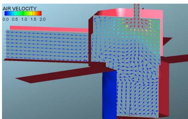
Fig. 5c Velocity vectors on a vertical plane through the centre of Tunnel 2, exit through top of tippel (empty bin scenario)
