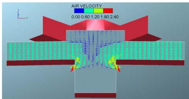
Fig. 4a Velocity vectors on a vertical plane through the centre of Tunnel 1 & 4, exit through 20 cm holes (empty bin scenario)
