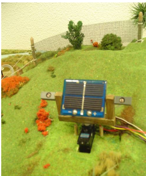
Figure 16: Tracking Solar panel
