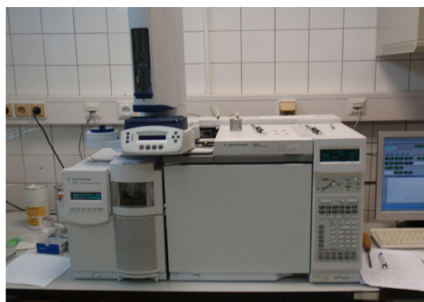
Fig. 1 Gas chromatograph with the mass detector
