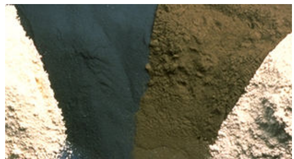
Fig.7 The colour of fly ash is variable from tan to black
