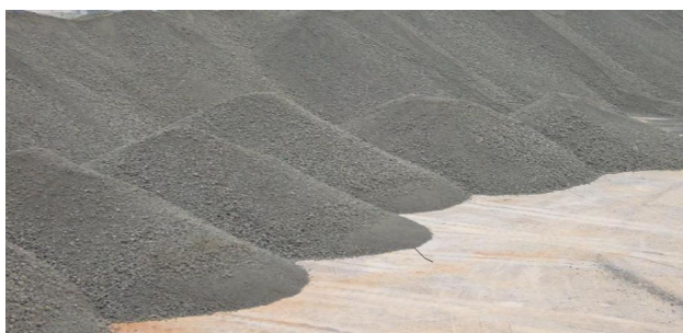
Fig.9 Dry storage of fly ash
