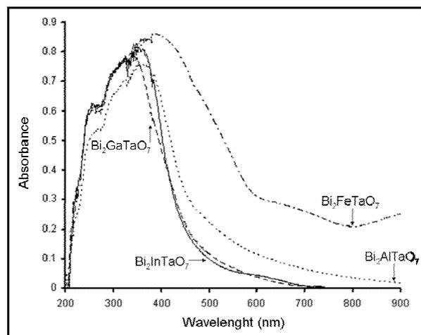
**Fig. 7.** UV-Vis spectra of solid state  $\text{Bi}_2\text{MTaO}_7$  ( $M = \text{Al, Ga, Fe or In}$ ).
