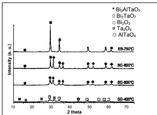
**Fig. 3.** XRD patterns of  $\text{Bi}_2\text{AlTaO}_7$  prepared by sol-gel and solid state reaction.
