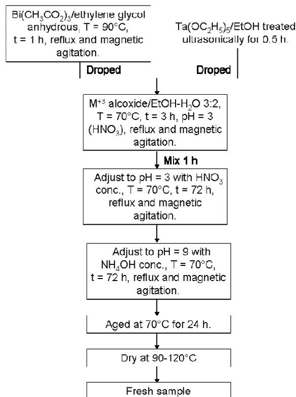
Fig. 1. Experimental diagram for the synthesis of pyrochlore compounds.
