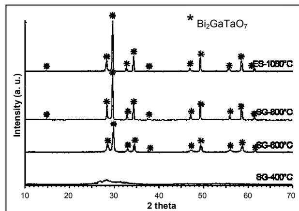
**Fig. 2.** XRD patterns of  $\text{Bi}_2\text{GaTaO}_7$  prepared by sol-gel and solid state reaction.
