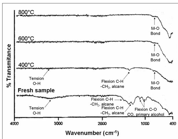
**Fig. 6.** FTIR spectra of sol-gel fresh sample for pyrochlore compound  $\text{Bi}_2\text{InTaO}_7$ .
