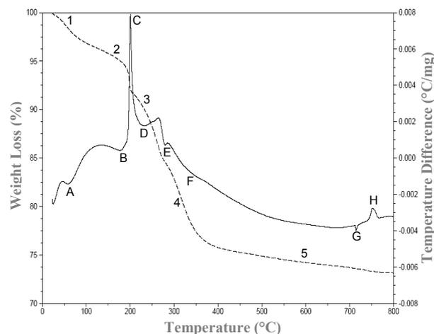
**Fig. 5.** DTA/TGA thermogram of sol-gel fresh sample for pyrochlore compound  $\text{Bi}_2\text{InTaO}_7$ .
