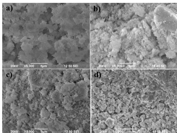
**Fig. 4.** SEM micrographs for pyrochlore compounds prepared by the sol-gel method at  $600^\circ\text{C}$ : a)  $\text{Bi}_2\text{GaTaO}_7$ , b)  $\text{Bi}_2\text{InTaO}_7$ , c)  $\text{Bi}_2\text{FeTaO}_7$ ; and by the solid state reaction at  $950^\circ\text{C}$ : d)  $\text{Bi}_2\text{InTaO}_7$ .
