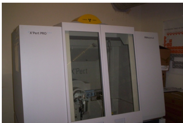
Fig.12 - PANalytical model X'Pert PRO with a detector of X'Accelerator equipment
