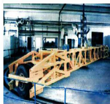
Fig.1 The ALT circular track facility of Technical University "Gh. Asachi" Iasi [3]
