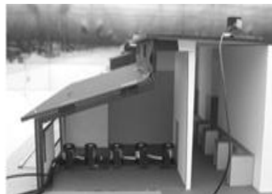
Figure 2. Flux metering equipment measuring the daylight factor
