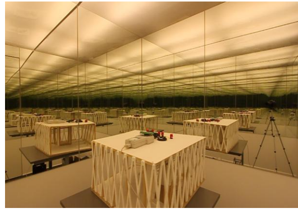
Figure 1. Overcast sky simulator interior view.
