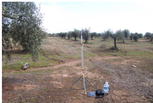
Figure 5- Measuring field saturated hydraulic conductivity to predict soil erodibility K factor (Used by permission of Thomas Panagopoulos ©2008, all rights reserved).
