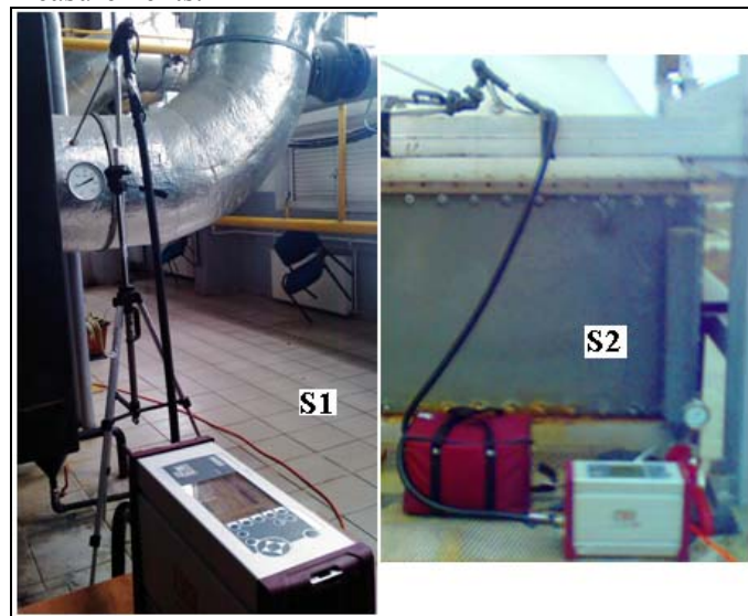
Fig.8 “Vario Plus” analyzer for emissions measuring at S1 and S2 sources
