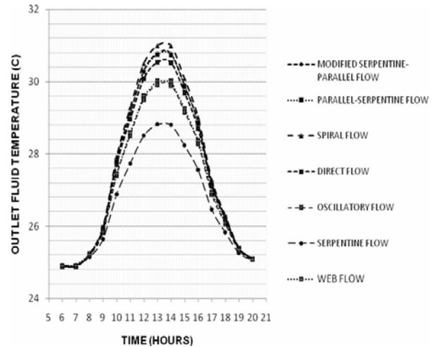
Fig.10 Variation of water temperature (output) versus the time of various absorber collectors
