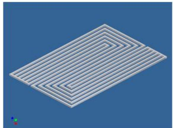
Fig.5: Parallel-Serpentine Flow Design
