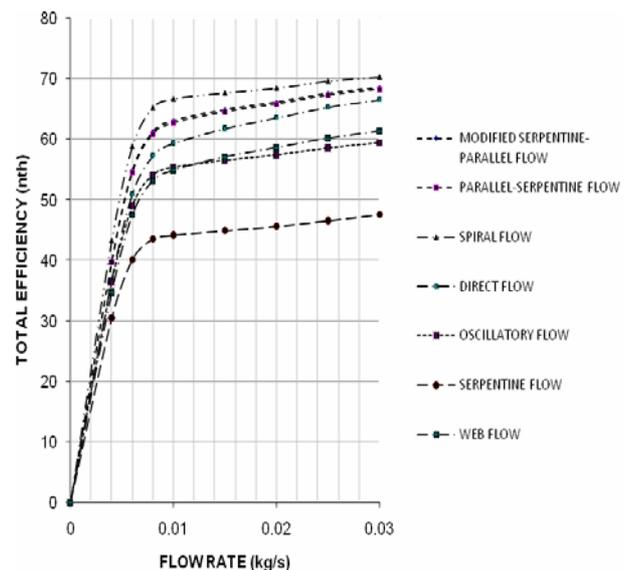
Fig.9 Flow rates configurations of various absorber collectors.
