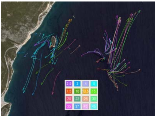
Fig. 3: The paths of the buoys in different depths during measurements (Depths are in meters)
