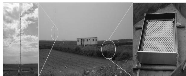
Fig. 2: Center: The experimental site. Left: the 20m meteorological mast. Right: the SODAR antenna.
