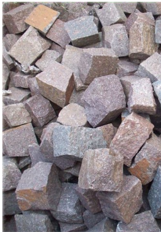
Fig.13: Material quarry. Porphyry cubes.
