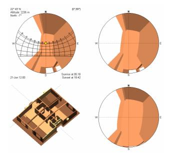
Fig. 5: Stereographic, equivalent (SF= 28.8%) and orthographic (SVF = 25.1%) projections
