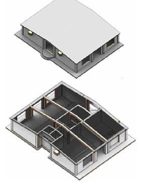
Fig. 6: With all its faces colored by the SVF, this building seems to be a renderized picture using the diffuse light produced by a clouded sky
