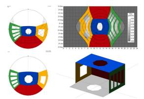
Fig. 7: Stereographic, isochronal and equivalent projection of a simple configuration
