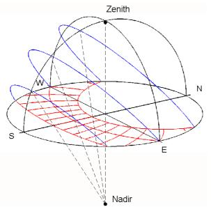
Fig. 1: Sun trajectories shown on the local hemisphere, and in the stereographic projection
