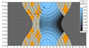
Fig. 3: Isochronal projection with superposed solar flux
