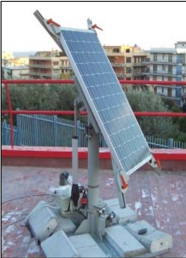
Fig. 3 Two axis tracking system
