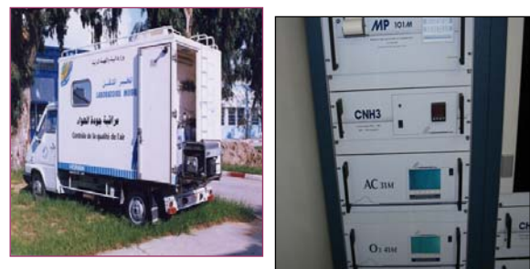
Fig.2: Mobile laboratory for air pollutants measurements and Acquisition systems of data.
