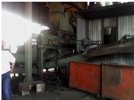
Fig. 7 Separation of ferrous metals from the others materials with a shredder Steinmertl equipment
