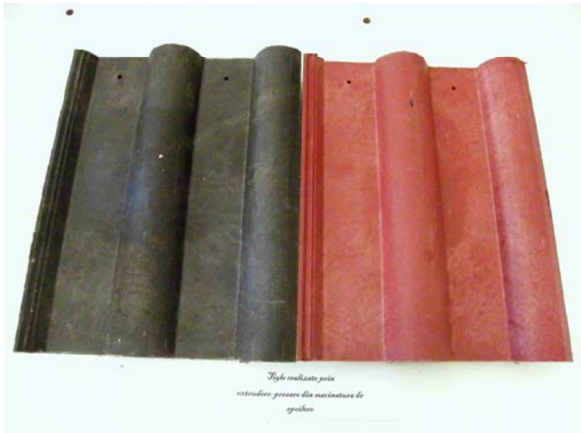
Fig. 15 Tiles from recovered polypropylene from ELV bumpers
