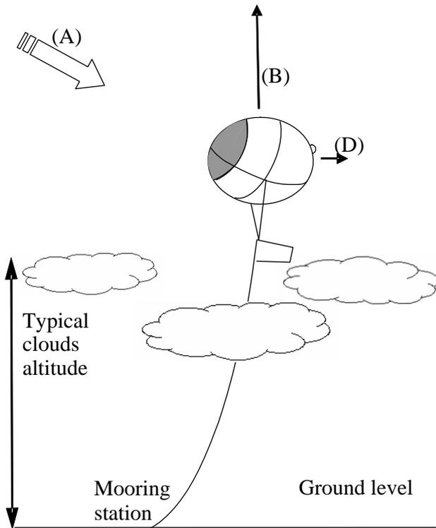
**Fig. 4: Schematic configuration of an Aerostat for Electrical Power Generation. The grey area represents PV cells cladding; B lift force (Buoyancy), D drag force, A solar beam direction**
