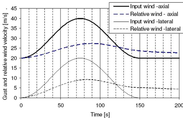
Fig. 10: Wind profile and relative wind velocity in the direction of the gust
