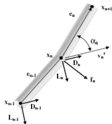
Fig. 8: Tether elements and wind vector
