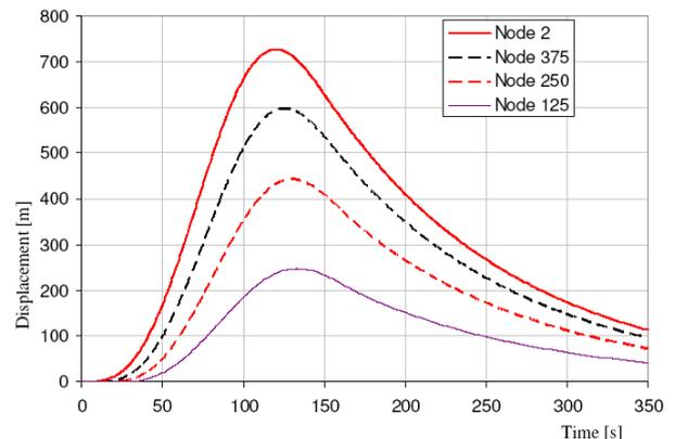
Fig. 12: Out of plane response of aerostat and tether line nodes subjected to a gust (20m/s, 150 sec duration) perpendicular to a constant wind (20 m/s)
