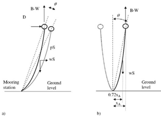
Fig. 9: Small oscillations a) with wind b) no wind
