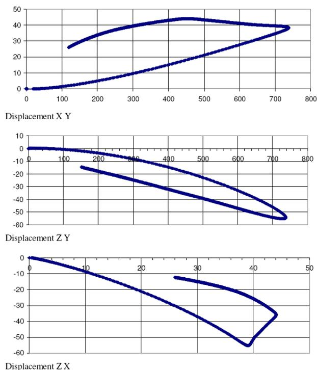
**Fig. 13: Trace of the aerostat displacements in the 3 planes, when subjected to a 20 m/s gust transverse to a 20 m/s constant wind speed**
