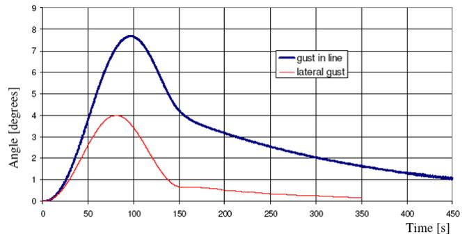
Fig. 11: Rotation of the aerostat produced by a 20 m/s gust summed to a 20 m/s constant wind speed
