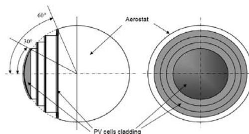
Fig. 6: PV cells cladding
