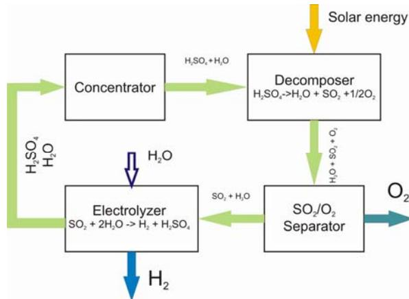
Fig. 2 Simplified schematic model of the WH cycle
