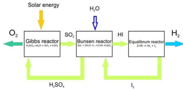
Fig. 3 Simplified schematic model of the SI cycle
