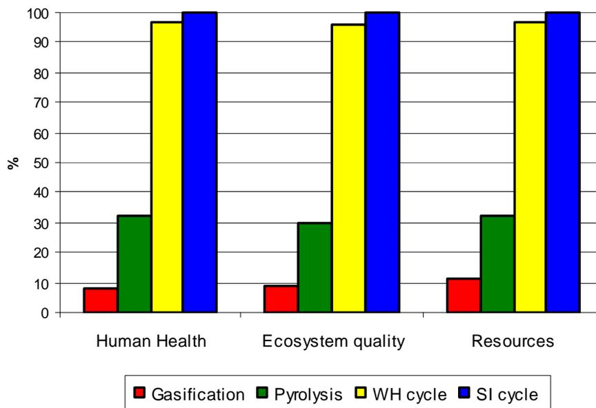
Fig. 5 Comparison of construction phase of WH cycle, SI cycle, gasification and pyrolysis
