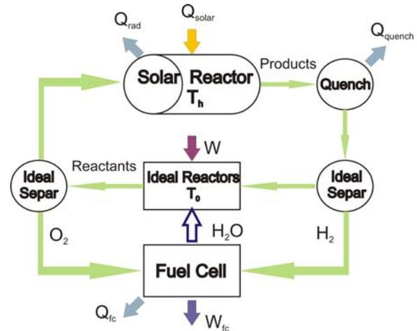
Fig. 1 Schematic model of solar energy conversion
