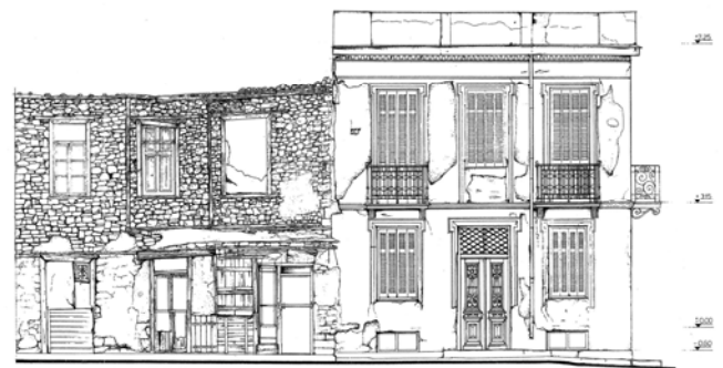
Fig.20 Thick masonry insulates the buildings from high temperatures.
