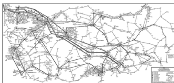
Fig. 2 Current Electricity Grid Lines in Turkey -2007
