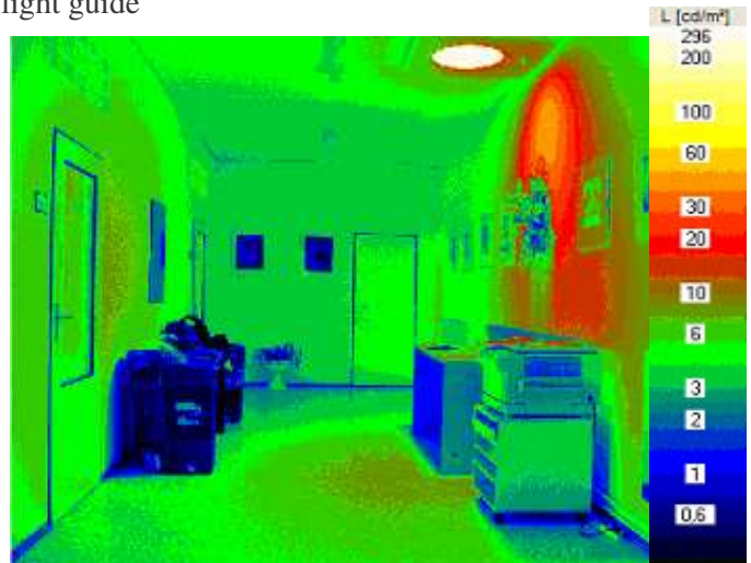
Fig. 8 Luminance photograph - luminance distribution inside of the room with the light guide (Luminance camera LMK)
