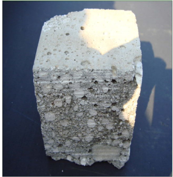
Figure 6: New recycled construction waste composite from lightweight concrete with aggregates with expanded glass and isolation waste from hard polyurethane
