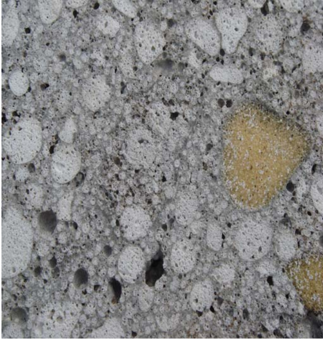
Figure 6: New recycled construction waste composite from lightweight concrete with aggregates with expanded glass and isolation waste from hard polyurethane
