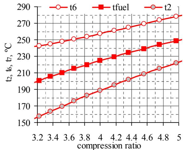
Fig.3  $t_2$ ,  $t_{fuel}=t_7$ , and  $t_6$  (biogas B,  $\theta=4.5$ ), vs.  $\epsilon$
