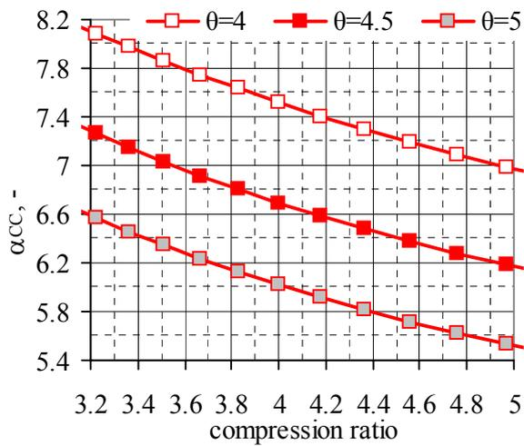
Fig.5  $\alpha_{CC}$  vs.  $\epsilon$ , for biogas B, and  $\theta=4$  to 5
