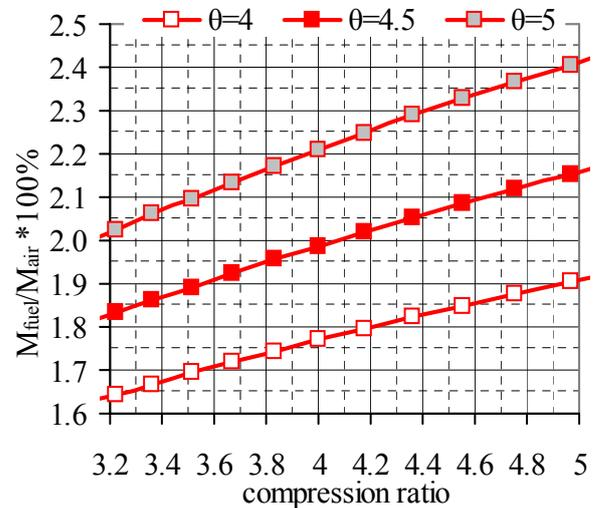
Fig. 19  $M_{fuel}/M_{air}$  vs.  $\epsilon$  for biogas B, and  $\theta=4$  to 5
