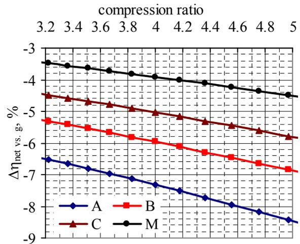
Fig.24  $\Delta\eta_{net\ vs.\ g}$  vs.  $\epsilon$  for  $\theta=4.5$ , all gases
