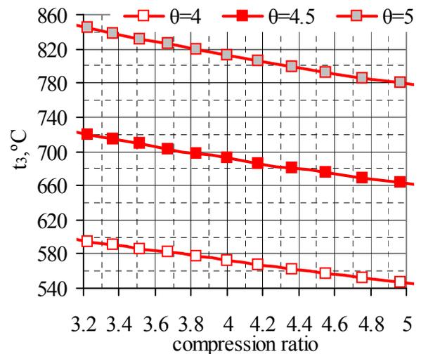
Fig.8  $t_3$  vs.  $\epsilon$ , for biogas B, and  $\theta=4$  to 5
