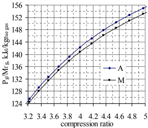
Fig. 15  $P_g/M_{f_g}$  vs.  $\epsilon$ , for M and biogas A,  $\theta=4.5$
