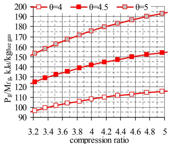
Fig. 14  $P_g/M_{fg}$  vs.  $\varepsilon$  for biogas B and  $\theta=4$  to 5
