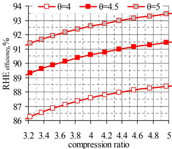
Fig. 11 RHE<sub>efficiency</sub> vs.  $\varepsilon$ , for biogas B, and  $\theta=4$  to 5
