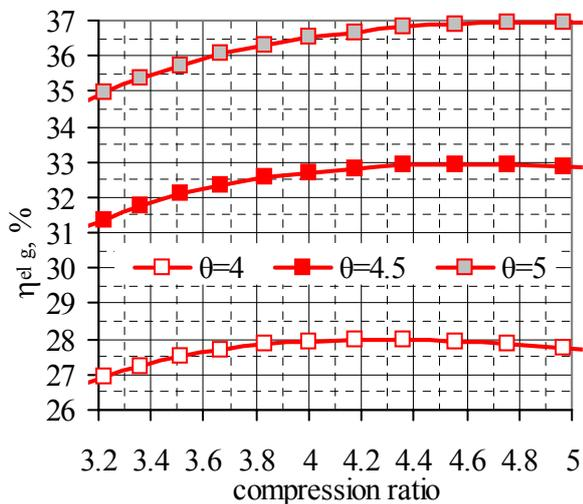
Fig. 16  $\eta_{el_g}$  vs.  $\epsilon$ , for biogas B, and  $\theta=4$  to 5
