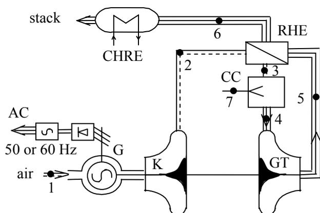
Fig.1 Single shaft micro gas turbine
