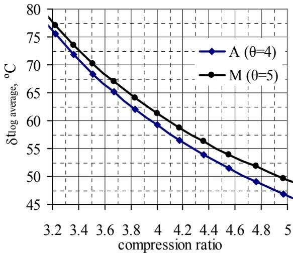
Fig. 10  $\delta t_{\log av}$  vs.  $\varepsilon$ , for biogas A ( $\theta=4$ ), and M ( $\theta=5$ )
