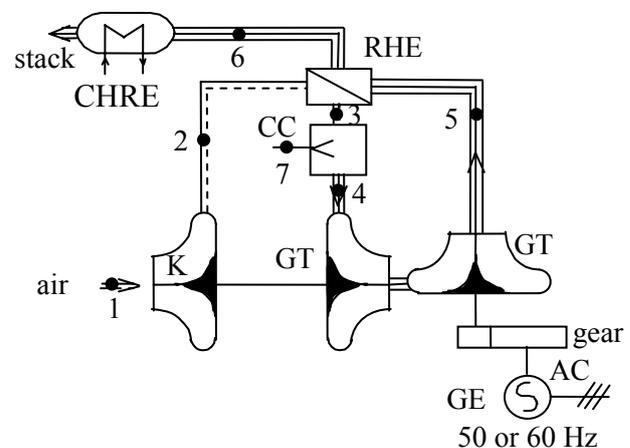
Fig.2 Double shaft micro gas turbine
