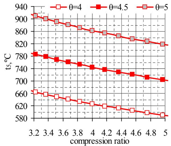
Fig.7  $t_5$  vs.  $\epsilon$ , for biogas B, and  $\theta=4$  to 5
