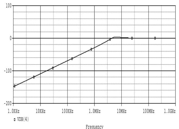
Fig. 4: Gain plot for high-pass filter.
