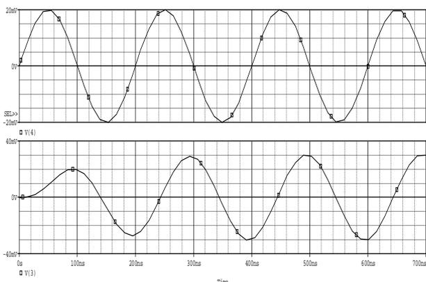
Fig.7: Input/Output low-pass waveforms at 5MHz.
