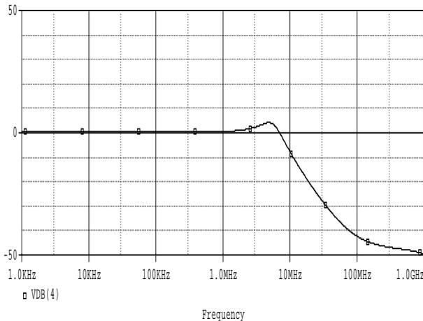
Fig. 6: Gain plot for low-pass filter.
