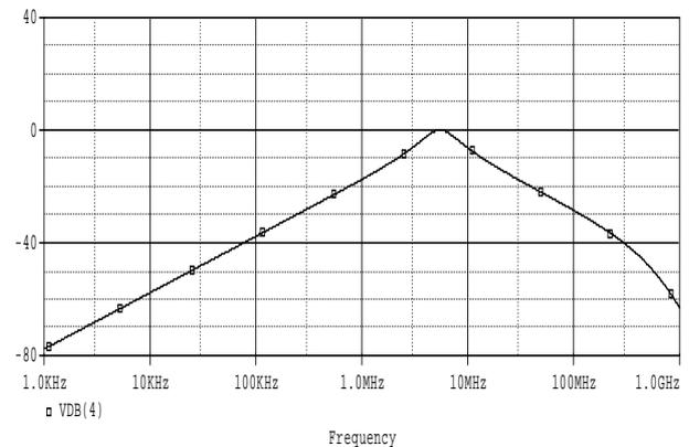
Fig. 3: Gain plot for band-pass filter.
