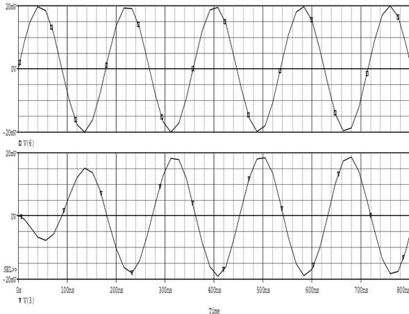
Fig. 5: Input/Output band-pass waveforms at 5.6MHz.
