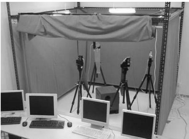
Fig. 8: Server Equipment: The server consists of four stereo cameras and five PCs. Camera and PC are connected through IEEE1394. The size of equipment is  $2.5(L) \times 2.5(W) \times 2.0(H)$  meters. The distance of target and each camera is about one meter.
