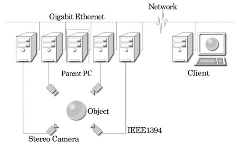
Fig. 1: Real Time 3D Imaging System: This is the client server system. The server acquires and transmits the 3D shape continuously. The client reconstructs and produces it. By repeating this procedure, it can generate the 3D sequence.
