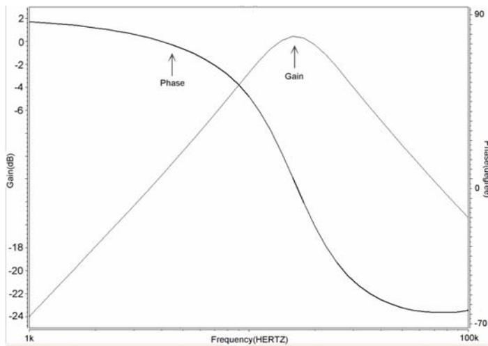
Fig. 18 Simulated frequency responses for the bandpass filter design with  $V_{in1} = V_{in3} = 0$  (grounded),  $V_{in2} = V_{in}$ .
