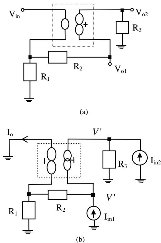
Fig. 7 (a) The plus-type nullor based amplifier.
