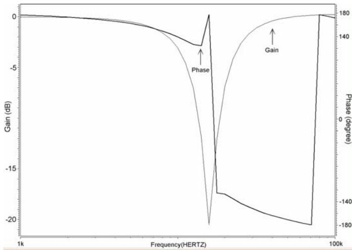
Fig. 20 Simulated frequency responses for the notch filter design with  $V_{in2} = 0$  (grounded),  $V_{in1} = V_{in3} = V_{in}$ .
