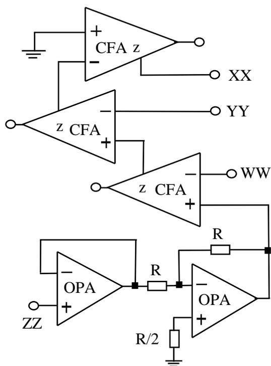
Fig. 14 The simulated circuit of ADJPN.
