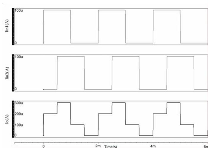
Fig. 15 The simulated input and output waveforms of Fig. 7.
