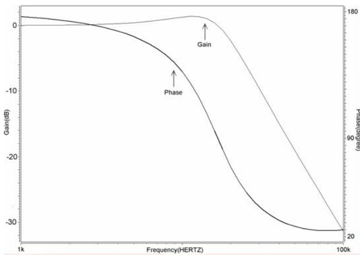
Fig. 19 Simulated frequency responses for the lowpass filter design with  $V_{in1} = V_{in2} = 0$  (grounded),  $V_{in3} = V_{in}$ .
