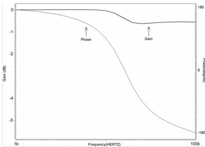
Fig. 21 Simulated frequency responses for the allpass filter design with  $V_{in1} = V_{in2} = V_{in3} = V_{in}$ .
