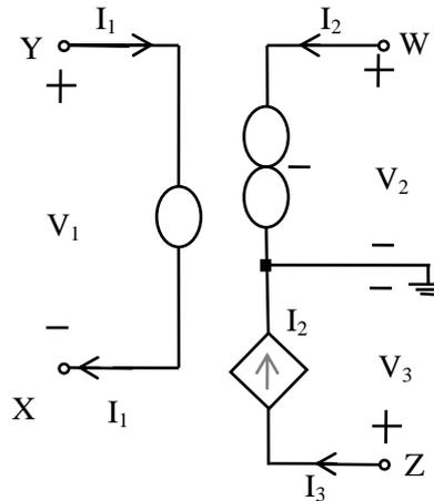
Fig. 3 An equivalent circuit of the plus-type nullor in Fig. 2.
