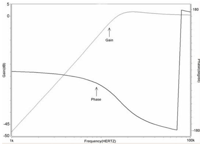
Fig. 17 Simulated frequency responses for the highpass filter design with  $V_{in2} = V_{in3} = 0$  (grounded),  $V_{in1} = V_{in}$ .
