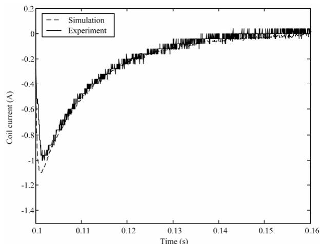
Fig. 12. Time-varying coil current curve during the opening process.
