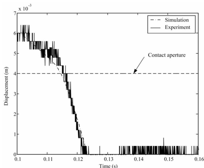
Fig. 13. Time-varying armature displacement curve during the opening process.
