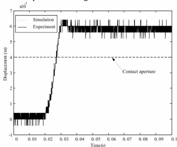
Fig. 10 Time-varying armature displacement curve during the closing process.
