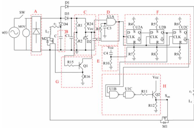
Fig. 5. Schematic diagram of completed electronic control unit (ECU).
