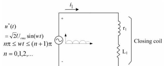
Fig. 2 The equivalent electrical circuit during the closing process.
