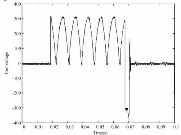
Fig. 7. Time-varying coil voltage curve during the closing process.
