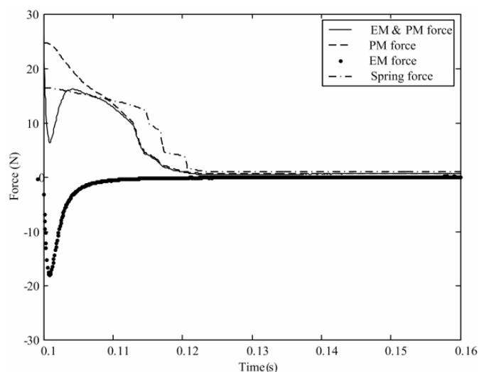
Fig. 14. Time-varying force curves during the opening process.
