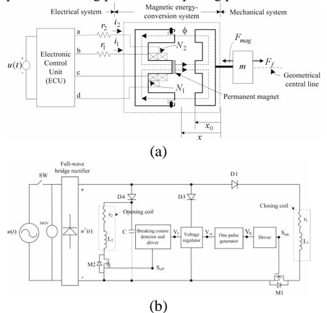
Fig. 1. Two sketches related to ac PM contactor, (a) mechanical structure (b) schematic block diagram of ECU.
