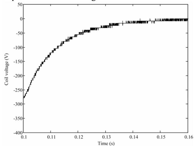
Fig. 11. Time-varying coil voltage curve during the opening process.
