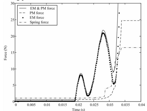
Fig. 9. Time-varying magnetic force curve during the closing process.
