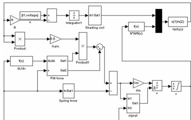
Fig. 6. Simulation model of proposed ac PM contactor model.
