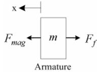
Fig. 4. Armature is viewed as a typical force-mass system.
