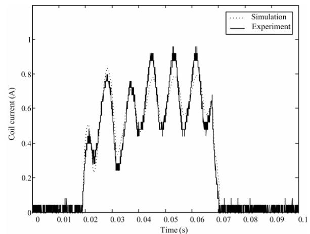
Fig. 8. Time-varying coil current curve during the closing process.
