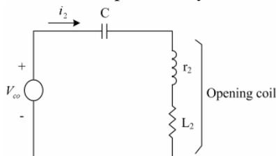
Fig. 3. The equivalent electrical circuit in the opening process.
