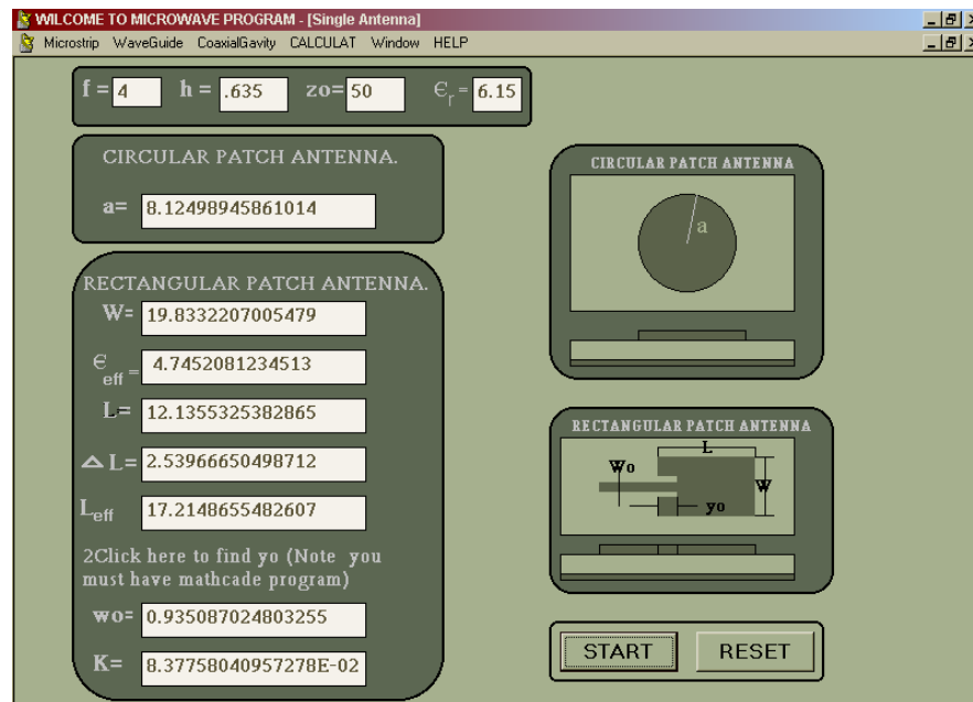
Fig. 8: The program entry, configuration and the basic calculations for single element MPA design
