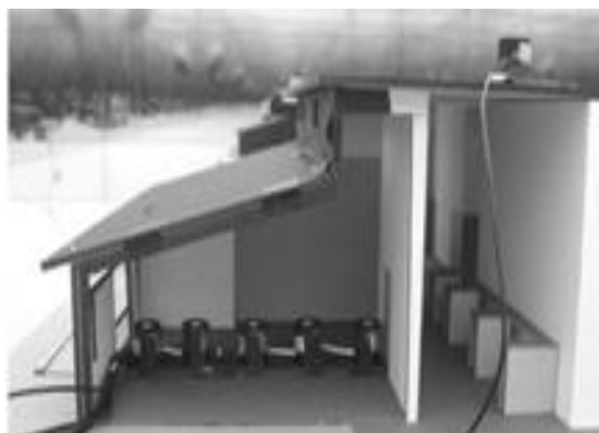
Figure 2. Flux metering equipment measuring the daylight factor
